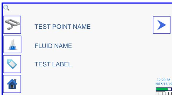
For example, if either the Test Point or Fluid buttons are pressed the screen will change to allow individual editing through buttons appearing to the right of the screen. Using the Test Label button will open the QWERTY keyboard.
