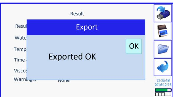
On a successful transfer a message box indicates the action is complete and also the number of tests transferred.
