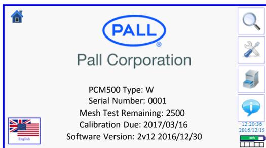
The main menu details PCM500 Type; Serial number; Remaining mesh test; Calibration due date, and software version.
